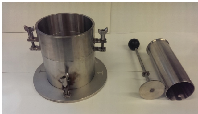
Figure 1.5.5.1.3.1 – Example of Proctor/Fagerberg test apparatus, hammer and hammer guide
