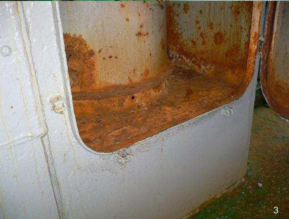
MV Atlantic Project: Unsafe hatch cover securing (1), corroded vent ducts (2, 3) and unsafe electrical installations (4)
