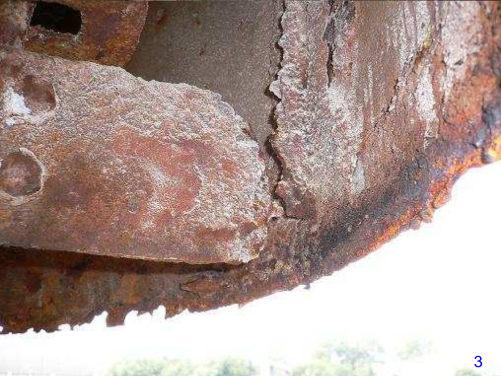
MV Evangelia: Excessive exhaust gas leakage in engine room (1) and lack of maintenance on deck (2), broken dampers for cargo hold vents (3, 4)
