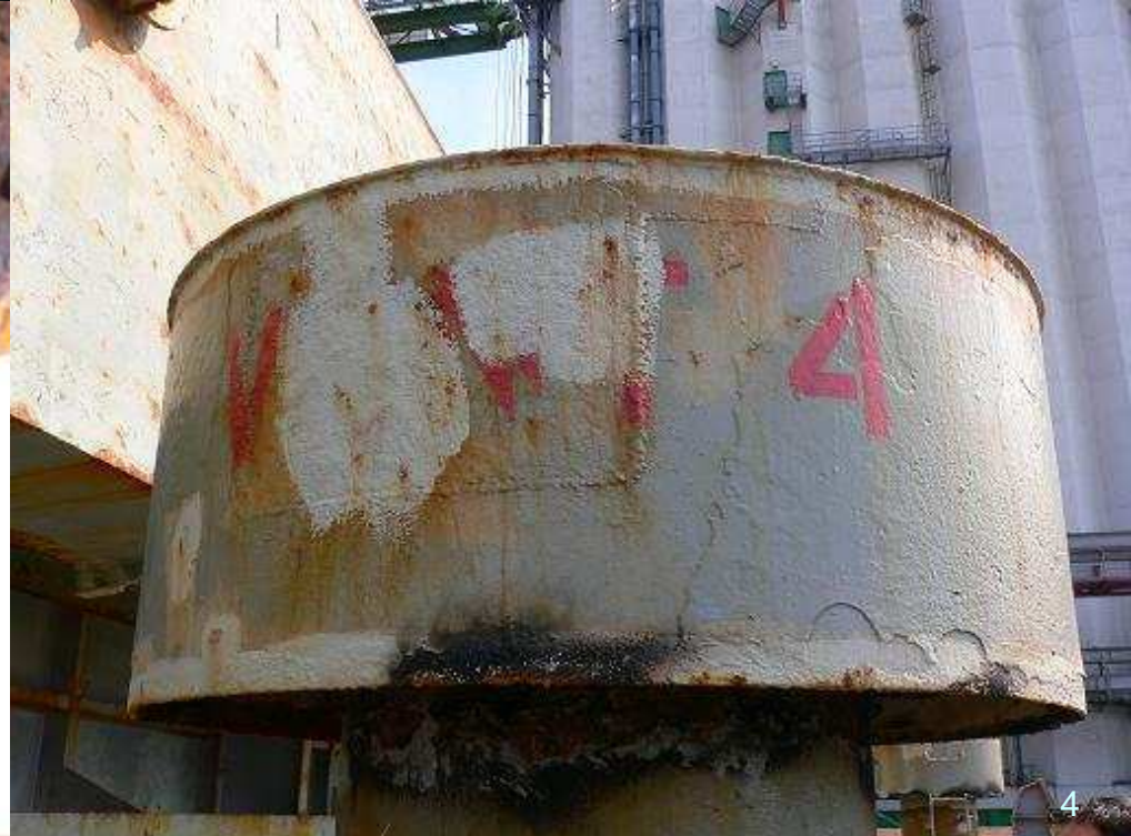
MV Evangelia: Excessive exhaust gas leakage in engine room (1) and lack of maintenance on deck (2), broken dampers for cargo hold vents (3, 4)
