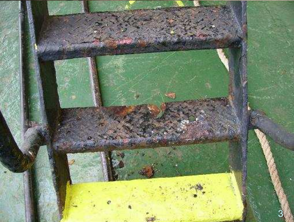
MV Vitafos: Damaged gangway (1, 2), corroded stairs (3) and damaged hatch cover sealing (4)
