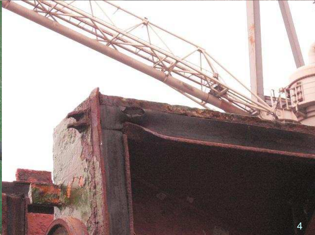
MV Vitafos: Damaged gangway (1, 2), corroded stairs (3) and damaged hatch cover sealing (4)
