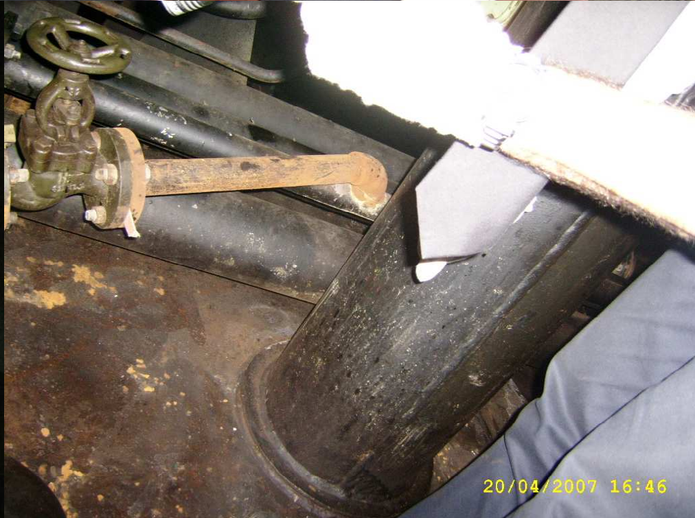
MV Zeynep Kiran: Sludge and bilgewater discharge via illegal bypass and bilge ejector into the sea
