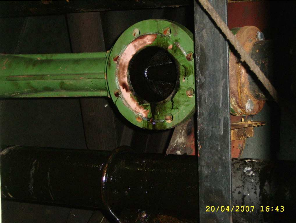
MV Zeynep Kiran: Sludge and bilgewater discharge via illegal bypass and bilge ejector into the sea
