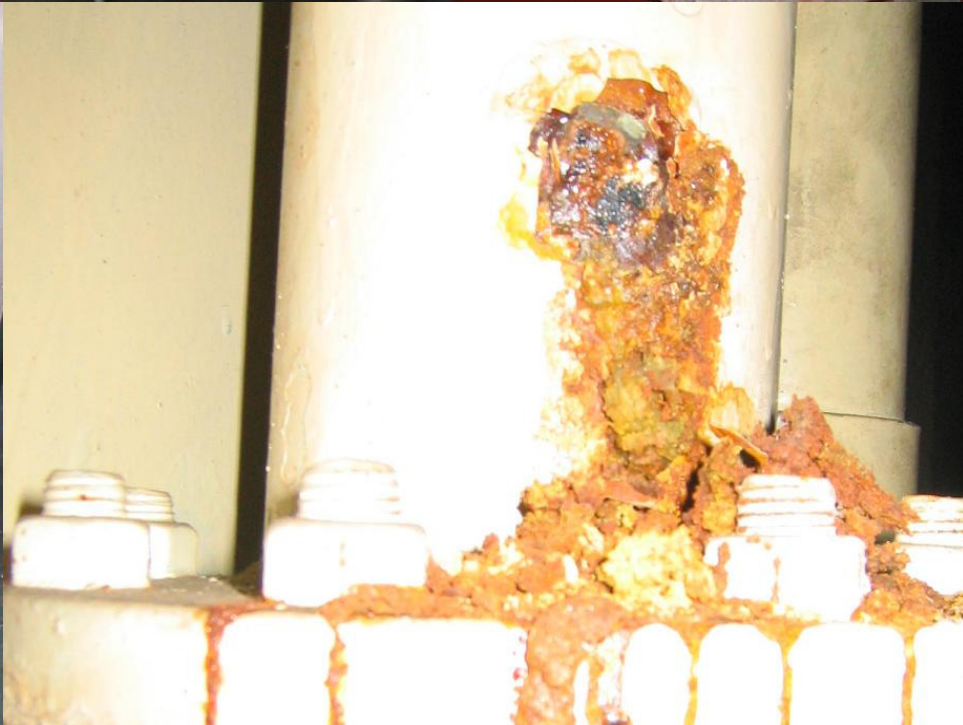
MV BSLE Pacific: mooring station obstructed, life boat damaged, oil leakages, overboard pipe corroded
