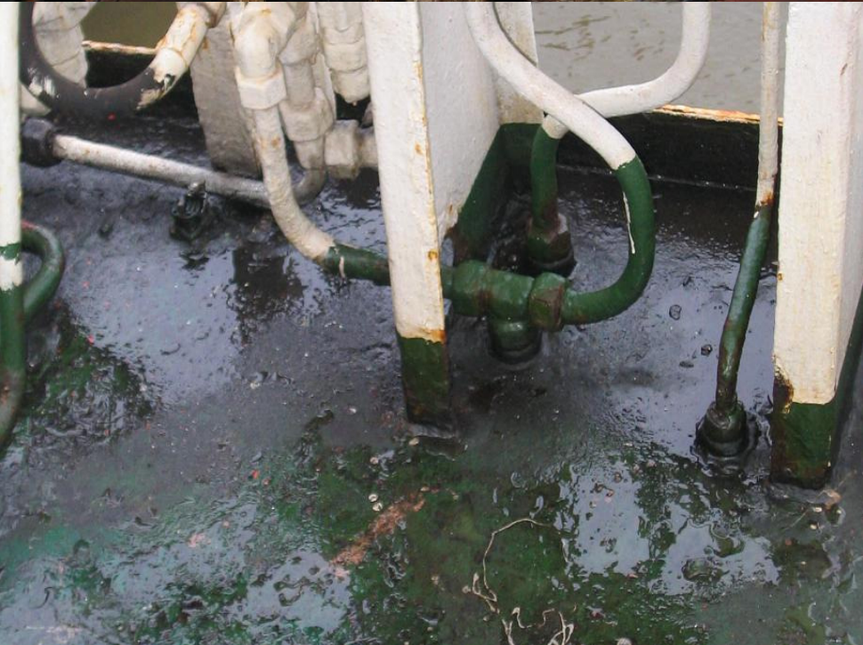
MV BSLE Pacific: mooring station obstructed, life boat damaged, oil leakages, overboard pipe corroded
