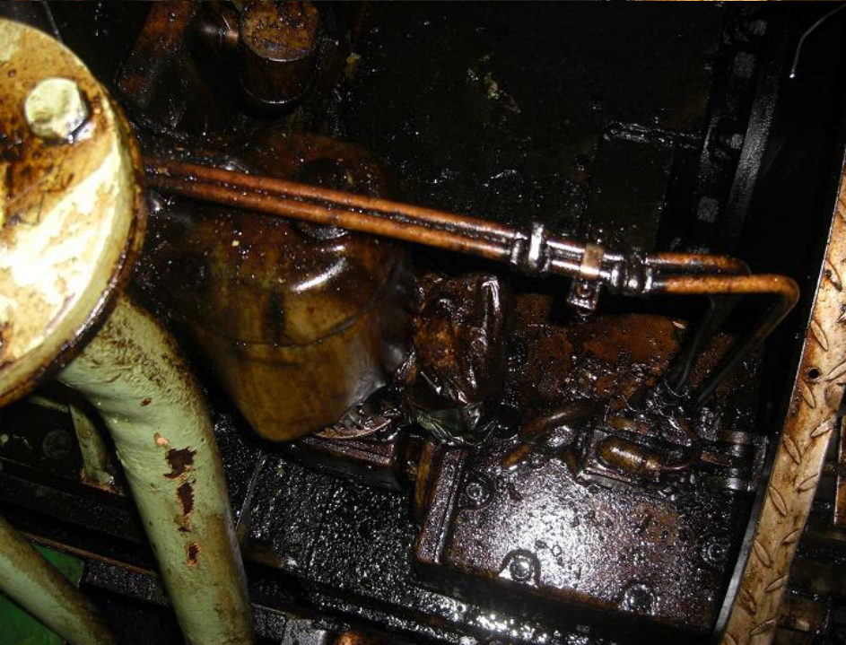
MV Lavina: oil leakages in engine room, poor maintenance
