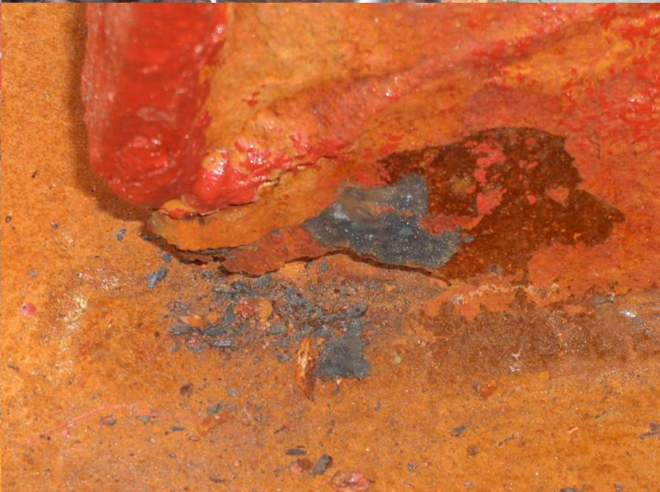
MV Red Cat: poor maintenance of life boat launching arrangement and release mechanism, corrosion and cracks on deck
