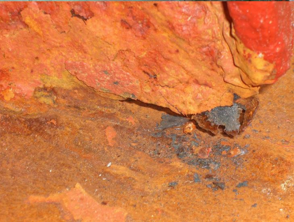
MV Red Cat: poor maintenance of life boat launching arrangement and release mechanism, corrosion and cracks on deck
