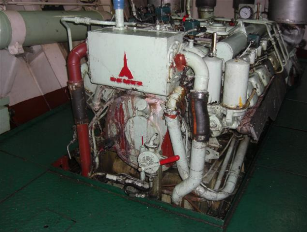
MV Djorf: poor maintenance of fire safety systems and deck equipment, also leakages at auxilliary engines, etc
