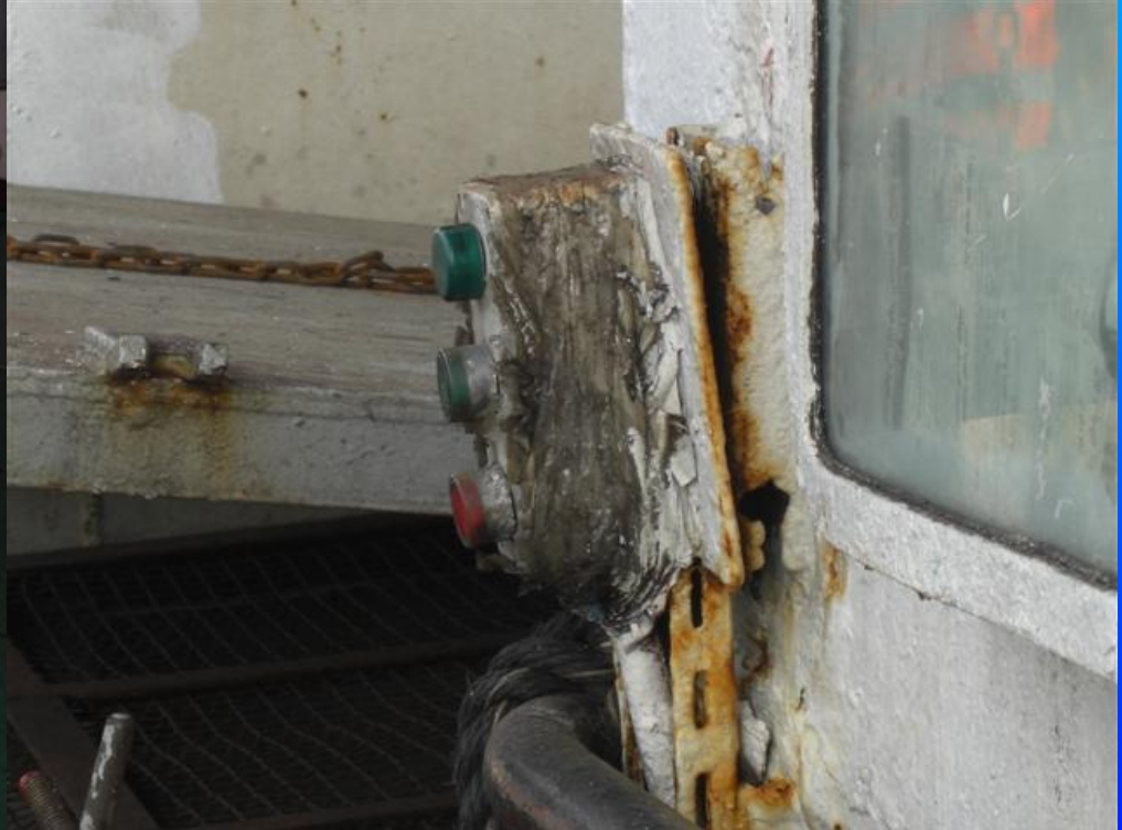
MV Djorf: poor maintenance of fire safety systems and deck equipment, also leakages at auxilliary engines, etc
