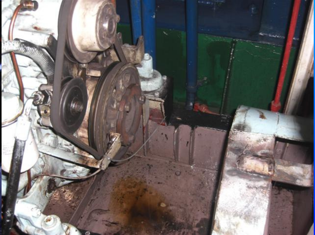
MV Maks: leakage from oil fired boiler, defective switches at boiler and fire pump, missing protection cover, etc
