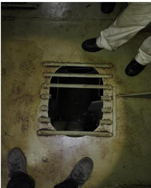
On this picture the fixed steel manhole cover for the bilge is broken. Nobody of the crew could explain why or when this had happened. In this dimly lit area a broken cover like this could lead to serious injuries.
