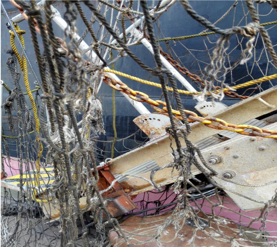
The first deficiency was already recorded when the PSCOs stepped on the gangway. The gangway net was fully worn out, with large gaps, comparable to a patchwork carpet. The picture speaks for itself
