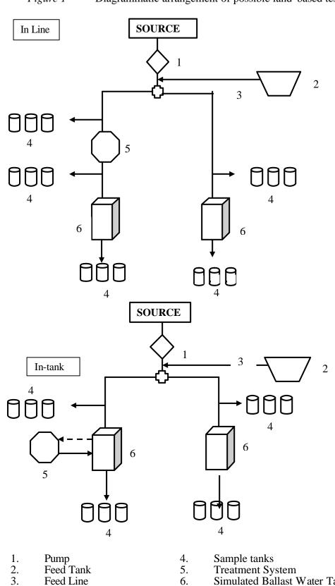
Figure 1 Diagrammatic arrangement of possible land-based tests
