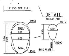
3 If a vertical opening is at a height of more than 600 mm steps then handgrips should be provided. In such arrangements it should be demonstrated that an injured person can be easily evacuated.
