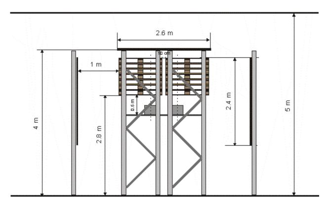
Figure 3.3.2.2 – End view of the cargo fuel package in a simulated truck
