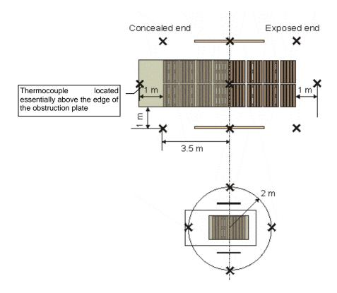
Figure 3.5.1 – Thermocouple locations in the two scenarios<sup>3</sup>
