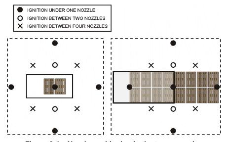
Figure 3.4 - Nozzle positioning in the two scenarios
