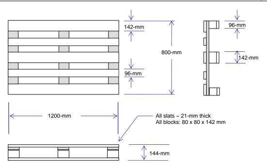
Figure 3.2.1 – Typical dimensions of the standard EUR pallet
