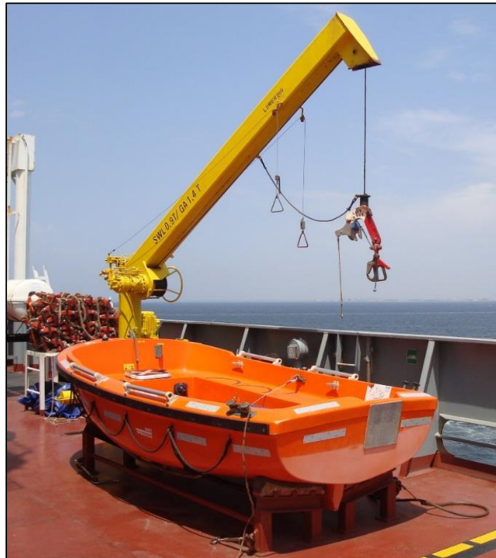
Figure 1: Launching appliance and rescue boat
