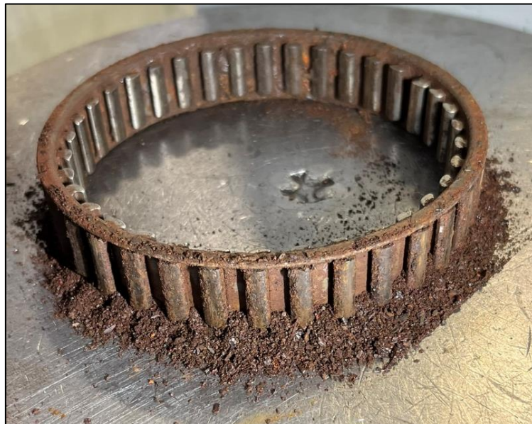
Figure 5: Freewheel after disassembly; traces of heavy corrosion on the sprags and sprag cage
