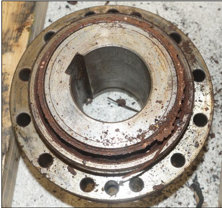
Figure 4: Weather-worn seal of the freewheel module
