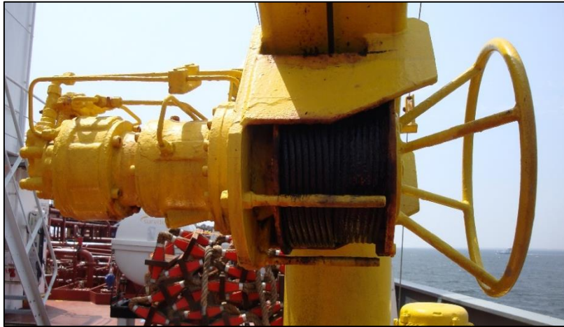
Figure 2: The launching appliance's winch unit
