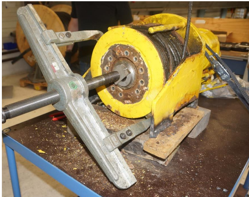
Figure 3: Disassembly of the winch unit
