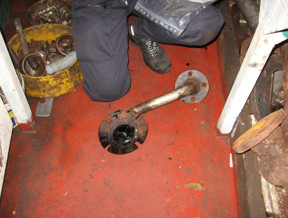
MV Kristi H: Sludge discharge via illegal connection to sewage system
