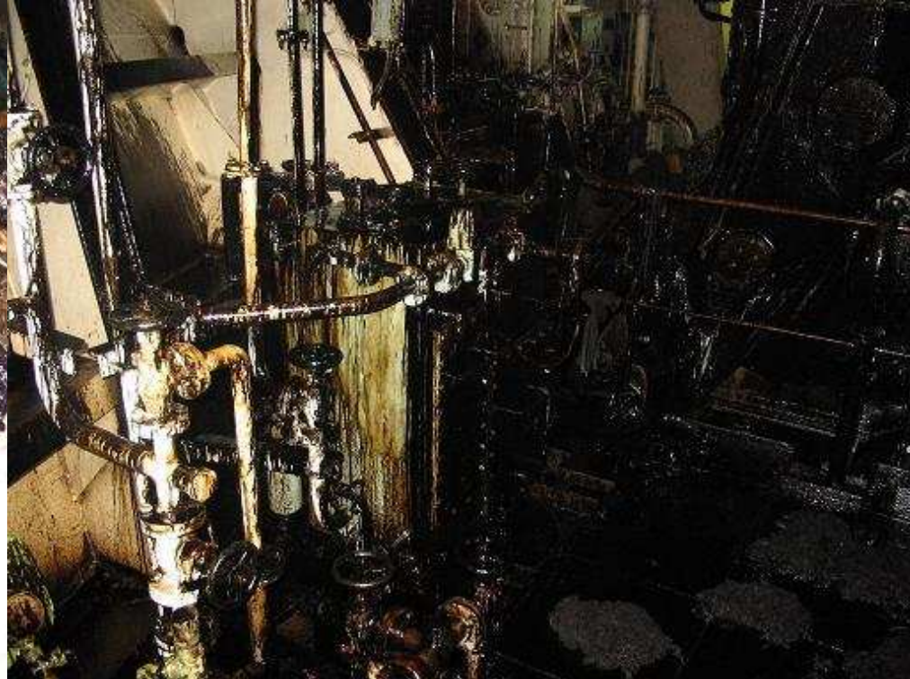
MV Bright Ruby: excessive amount of waste oil in engine room bilges, engine room totally spoiled
