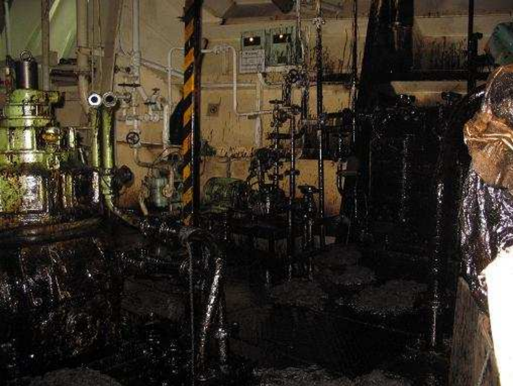
MV Bright Ruby: excessive amount of waste oil in engine room bilges, engine room totally spoiled
