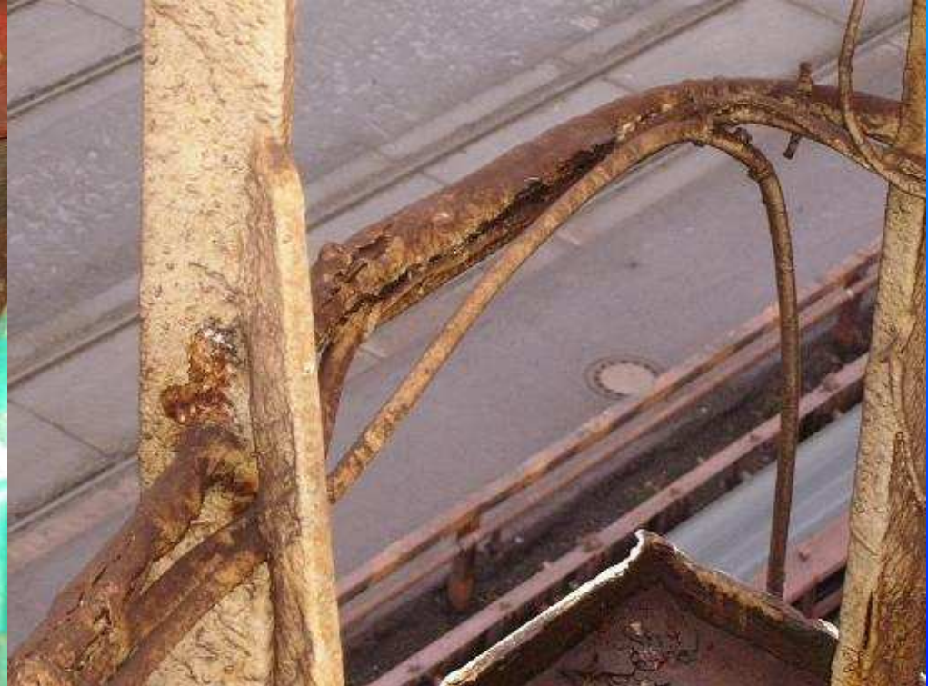
MV EEC Atlantic: broken fire line, deck corroded through, corrosion at seachest, insufficient maintenance on deck, etc.
