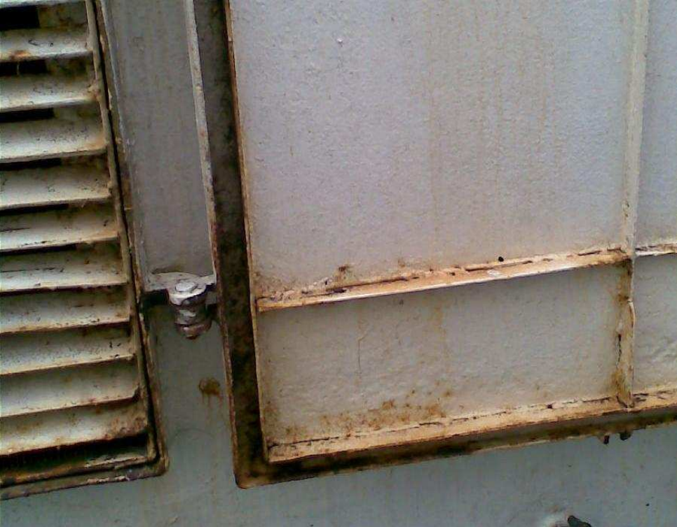
MV Skarven: insufficient deck maintenance, crack and holes in superstructure, fire dampers in bad condition or missing, etc.
