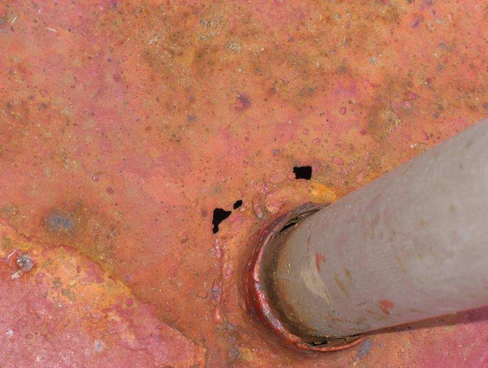
MV Baltic Wind: Decks corrosion, cracking, damaged hatch cover, broken hinges at watertight door, etc.
