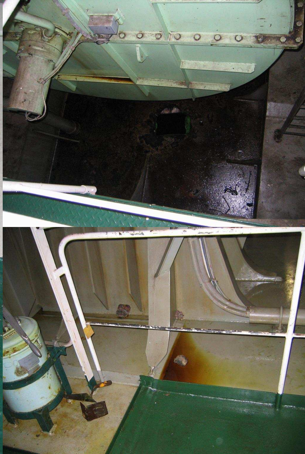
MV CMA CGM Berlioz: Temporary repair at overboard valve not properly carried out, oil leakages in E/R, etc.
