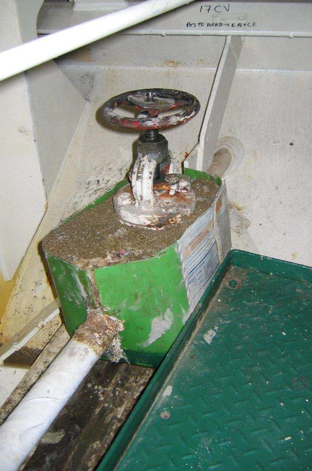
MV CMA CGM Berlioz: Temporary repair at overboard valve not properly carried out, oil leakages in E/R, etc.
