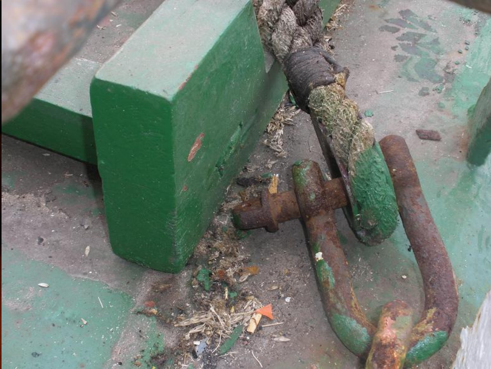
MV Dana-1: unhygienic refrigerator, no safety shoes during boat drill, unsafe shackle for embarkation ladder
