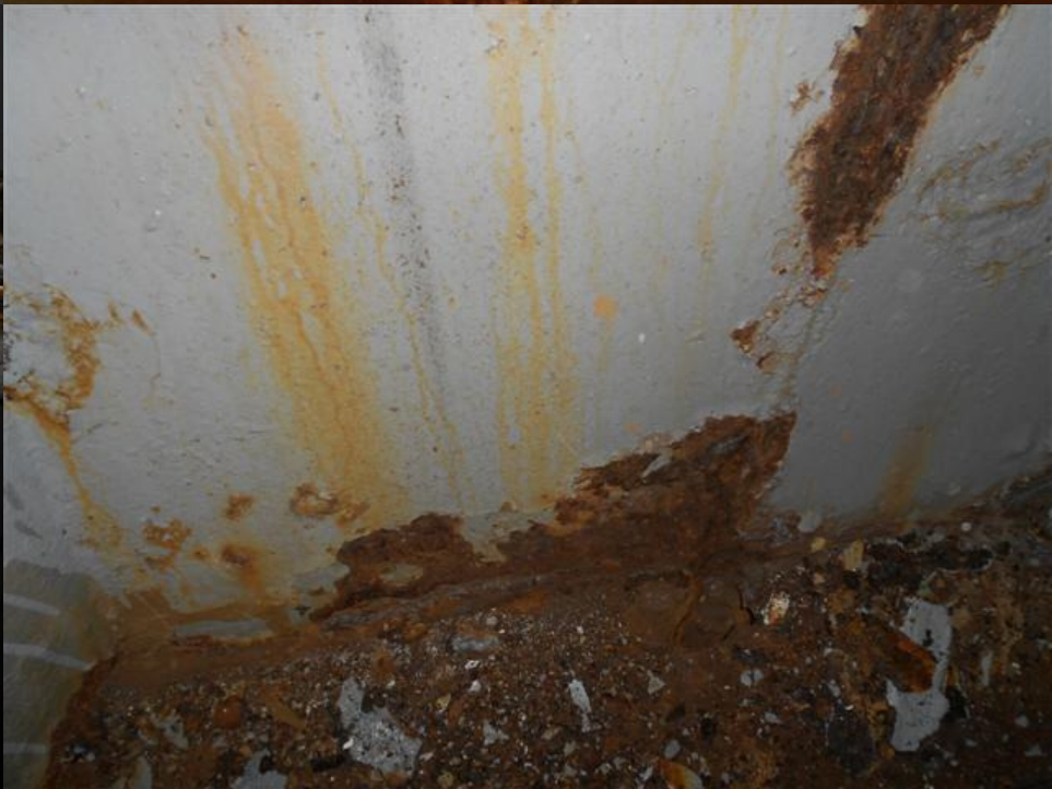
MV Rasim Akar: poor maintenance on deck and in engine room, excessive corrosion on engine room hull plating
