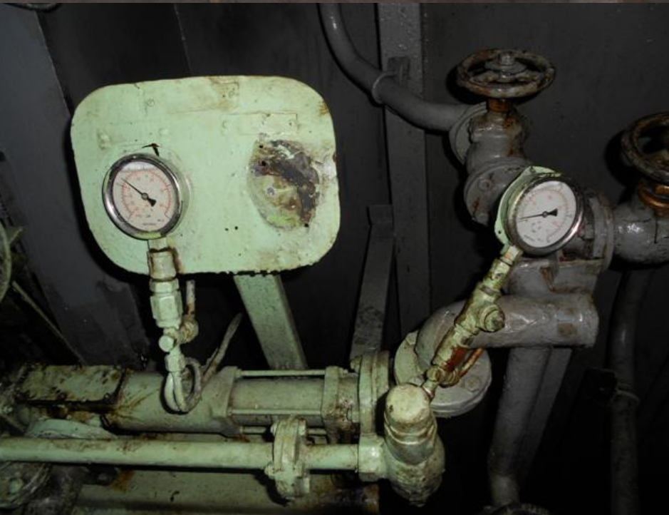
MV Rasim Akar: poor maintenance on deck and in engine room, excessive corrosion on engine room hull plating
