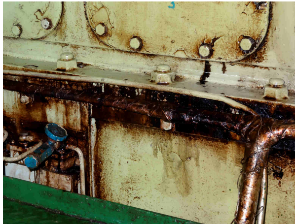
picture 19: insulations wetted through oil
