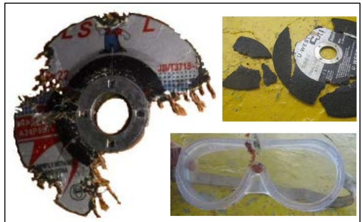
Shattered cutting disc
